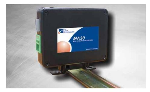
With a unique 'three-stage' combination of protection elements, these units suppress conducted RFI and voltage surges. The circuit elements are first, surge clipping components to absorb transient surges that may otherwise damage equipment; second a filter to suppress noise in the system and third, 'ring' suppression. The third of these prevents surges causing the filter to 'ring' (oscillate) under low load conditions – an
